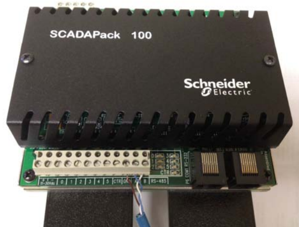
Figure 21 - SCADAPack 100 With Attached CAT5E Cable
